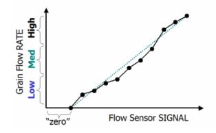
Other manufacturers recommend between 3 and 6 grain loads to perform a satisfactory calibration of the yield monitor. This suggests that the calibration response curve for these yield monitors is not a straight-line, but is rather some sort of non-linear response curve that requires a number of calibration points to best "train" the yield monitor how to interpret the flow sensor signals.
